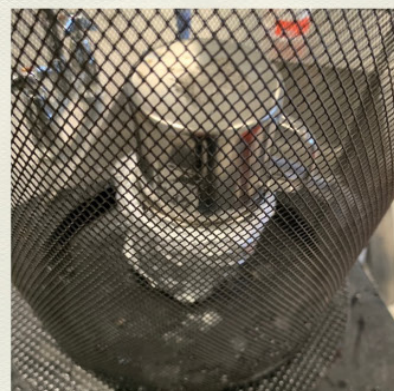
24. Use a second metallic cup to suffocate the fire and leave in place until fire is extinguished
