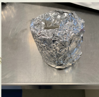
7. Wrap the dish and cup with alfoil (do not wrap it over the bottom of the cup)
