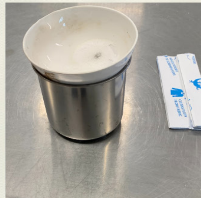
6. Place Evaporating Dish on top of cup
