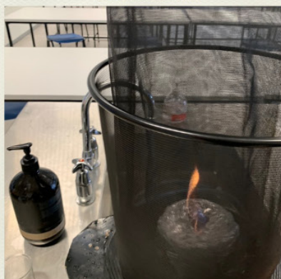
23. When the rotation slows down, the flame will reduce
