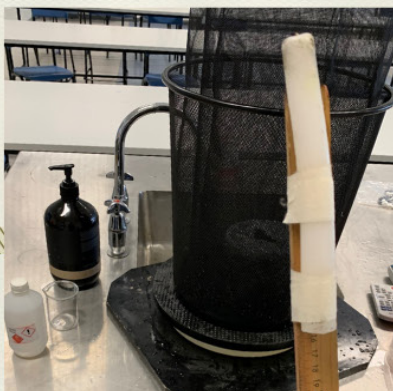
19. Attach a candle or taper to the end of a long stick or 1m ruler
