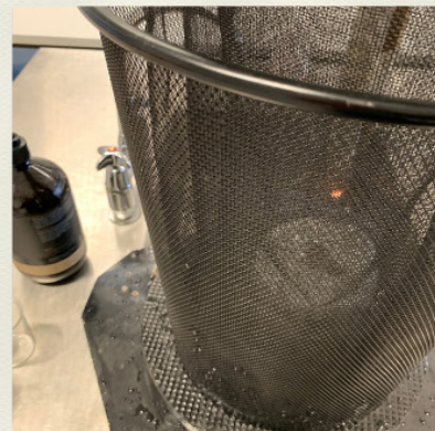
18. Place fine wire mesh (i.e. fly screen) into bin so that it surrounds the equipment inside
