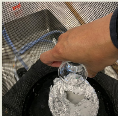
17. Carefully pour flammable liquid into the Evaporating Dish containing the salt.
