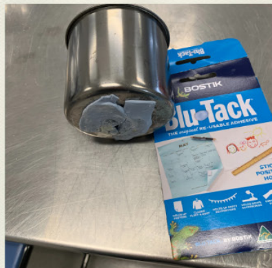
5. Add some Blu-Tack to bottom of one metal cup
